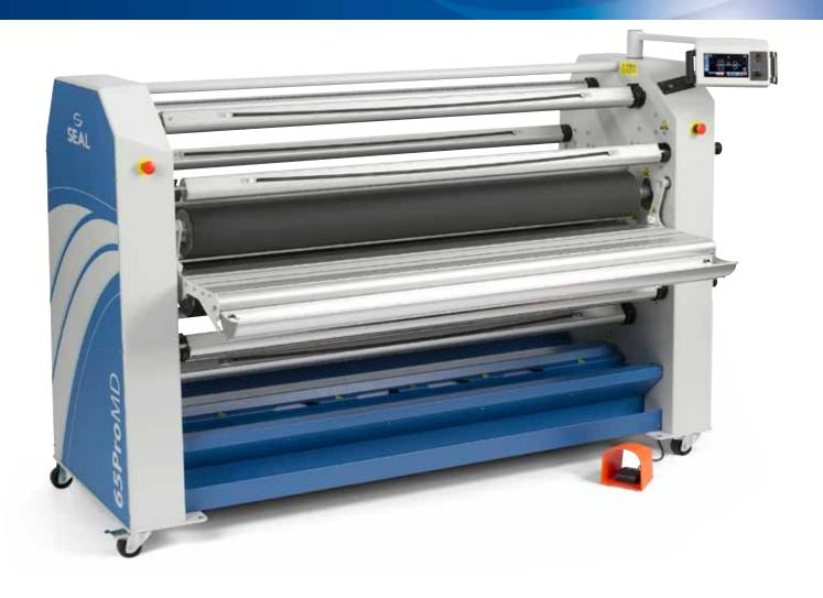
The SEAL 65 Pro MD is a fully featured, high performance laminator for a high performance environment. This dual heated, bi-directional, pneumatically operated machine will mount, laminate and encapsulate a wide range of materials and substrates up to 1650 mm wide and 50 mm thick and is particularly suited to the extensive range of SEAL consumables.
